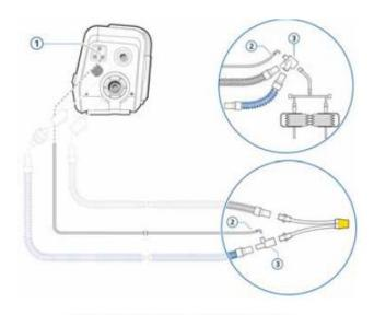
Figure 6-8. Connecting the pressure line
