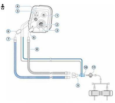
Figure 6-5. MR Safe dual-limb breathing circuit with HMEF/HME for use in MRI environment (neonatal)
