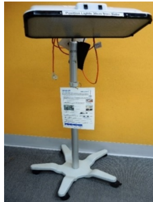
Figure 6: Natus Neoblue freestanding unit (Picture from NICU, JHCH)
