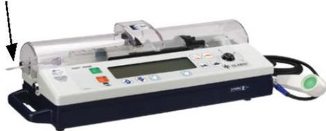
flanges touch the front of the slot closest to the syringe tip. This action will prevent delay at the start of the treatment. Rotate the syringe clamp anticlockwise until it locks onto the syringe barrel
