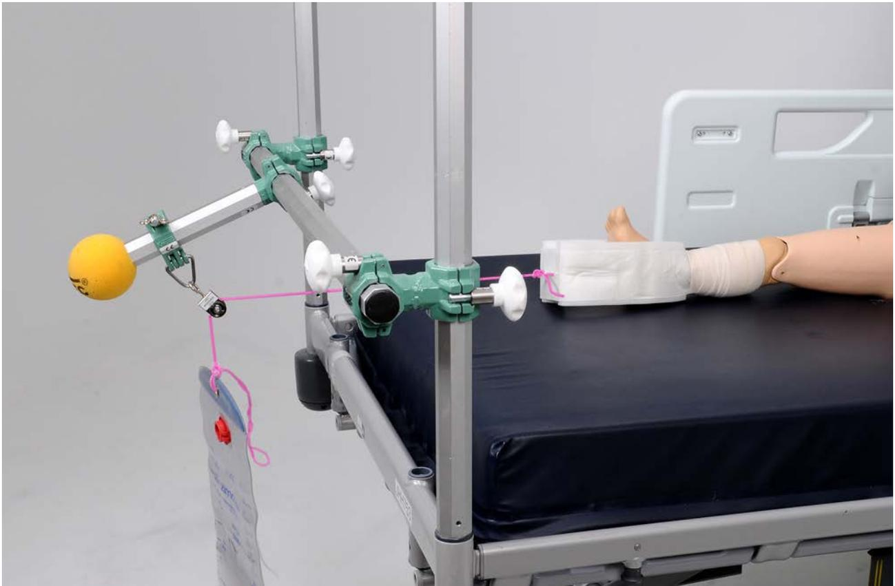
Figure 8. The rope is threaded through a pulley and the weight bag hangs at a 90° angle.
