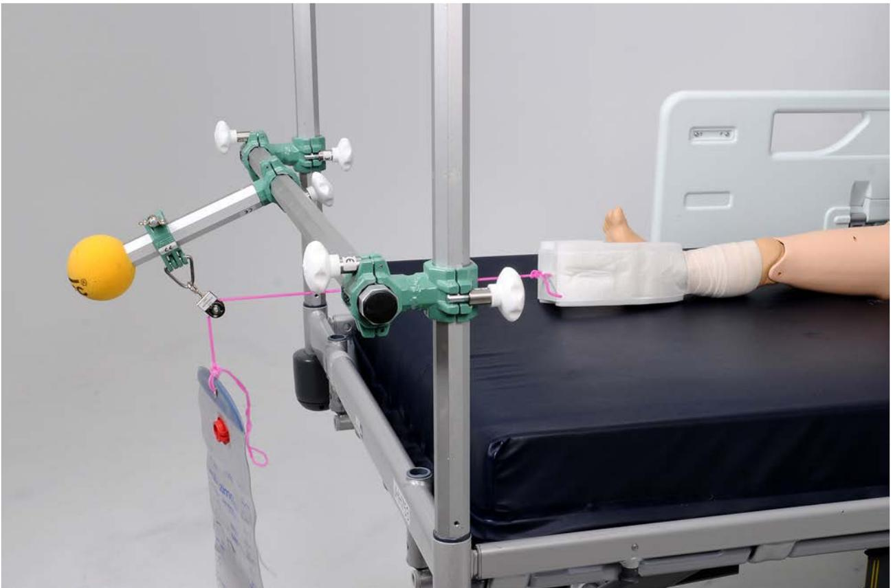
Figure 7. The rope is threaded through a pulley and the weight bag hangs at a 90° angle.
